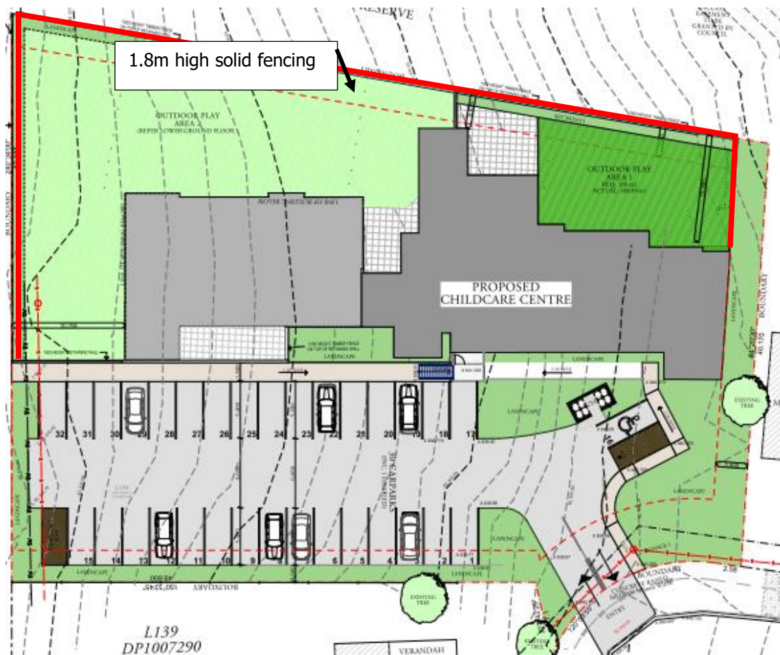
Figure 6-1 Site boundary fences to mitigate external traffic noise
